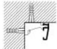
Screw for wall or ceiling with universal bracket.
