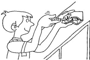
Firmly screw **3175** brackets to wall or ceiling. The two outside brackets should be located 10cm (4") in from the ends of track so as not to coincide with end covers. Remaining brackets should be equally spaced along track (approx. every 30-50cm/12"-20').
