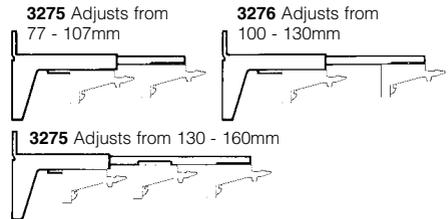
Up to 3 tracks can be located on the same extension bracket or a pelmet formed around your existing track.
